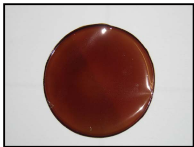
Figure 2. Porphyrinated cellulose laurate plastic film of 0.52% PpIX content.
